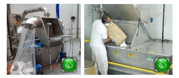
Figure 7. Examples of dumping stations.
