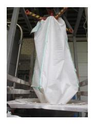
Figure 13. Sealing system for big bag discharging purpose.
