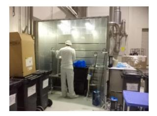
Figure 5. Examples of (pre-) weighing units for enzymes.
