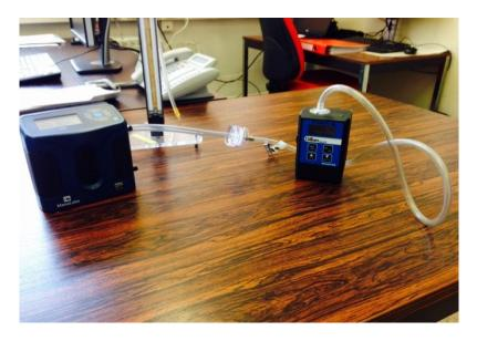
Figure 32. Calibration set-up for air sampling equipment.
