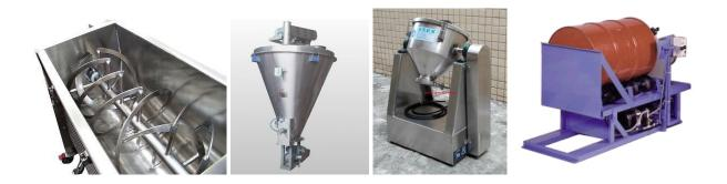
Figure 6. Examples of industrial blending stations for bakery improvers & mixes.
