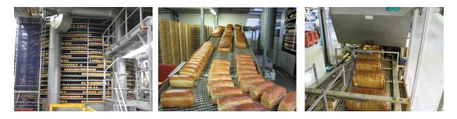
Figure 16. Conveying final product in industrial bakeries.
