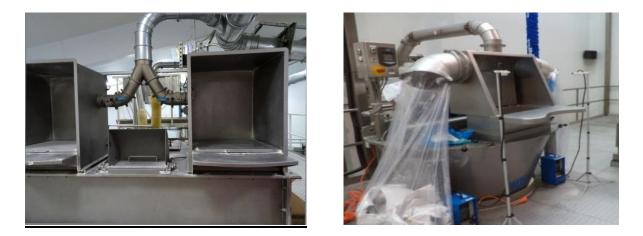
Figure 9. Ventilation principles for paper bag emptying operation (preferably through the back of the unit).
