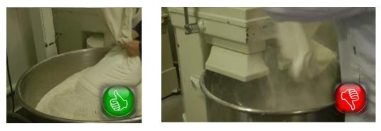
Figure 19. Unloading flour and improvers in mixing bowls: dos and don'ts.
