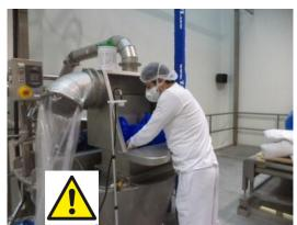
Figure 8. Type of respiratory mask only suitable for low-risk operations based on the results of the risk analysis.
