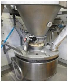
Figure 14. Connection system for silos.
